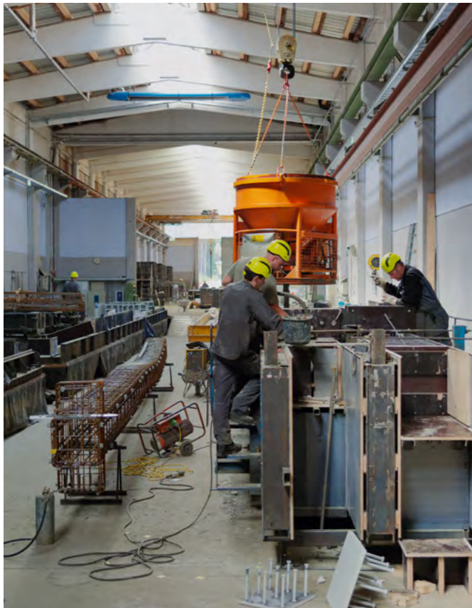
Production of Leube noise-protection walls at the plant in Maishofen
